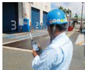
(1) Regular measurement with an odor measurement device
